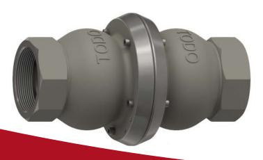
The TODO NGX Break-Away Coupling has been designed to eliminate spillage and damage associated with drive and/or pull away incidents. The coupler identifies an excessive load, closes the valves and then allows for disconnection.
