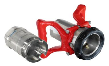
The TODO-GAS™ couplings are designed primarily for loading/ unloading of railcars, bobtails and intermediate bulk delivery trucks. A release upon disconnection volume of only 0.35 cc and with one or two handle options and an integral swivel, TODO-GAS™ 2" couplings can cope with almost any loading equipment.
