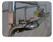
Parallel deviceto keep the filling tube horizontal all the time.
